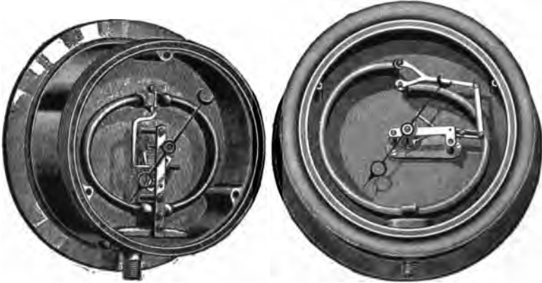
ASHCROFT STEAM GAUGE. CROSBY STEAM GAUGE.
